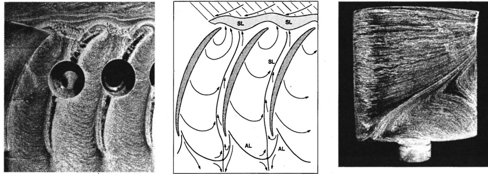
Fig. 10 Oil flow picture of stator A at part load ( \varphi=0.37 ) on stator hub and suction surface
