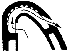
Fig. 1 Turbine blade cooling passage with hemispherical surface dimples in a leading edge area (concave wall; possible design)
